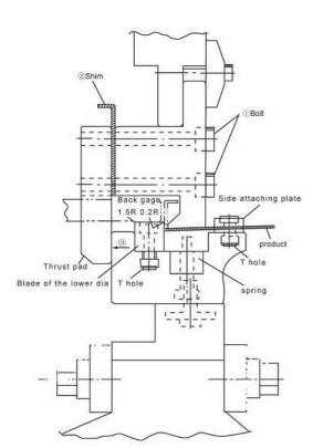
First, adjust the clearance of upper and lower dies according to the thickness of the material to be bent.
